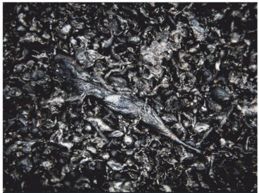
Extract from Redwood Materials' furnace, which melts down lithium batteries for recycling
